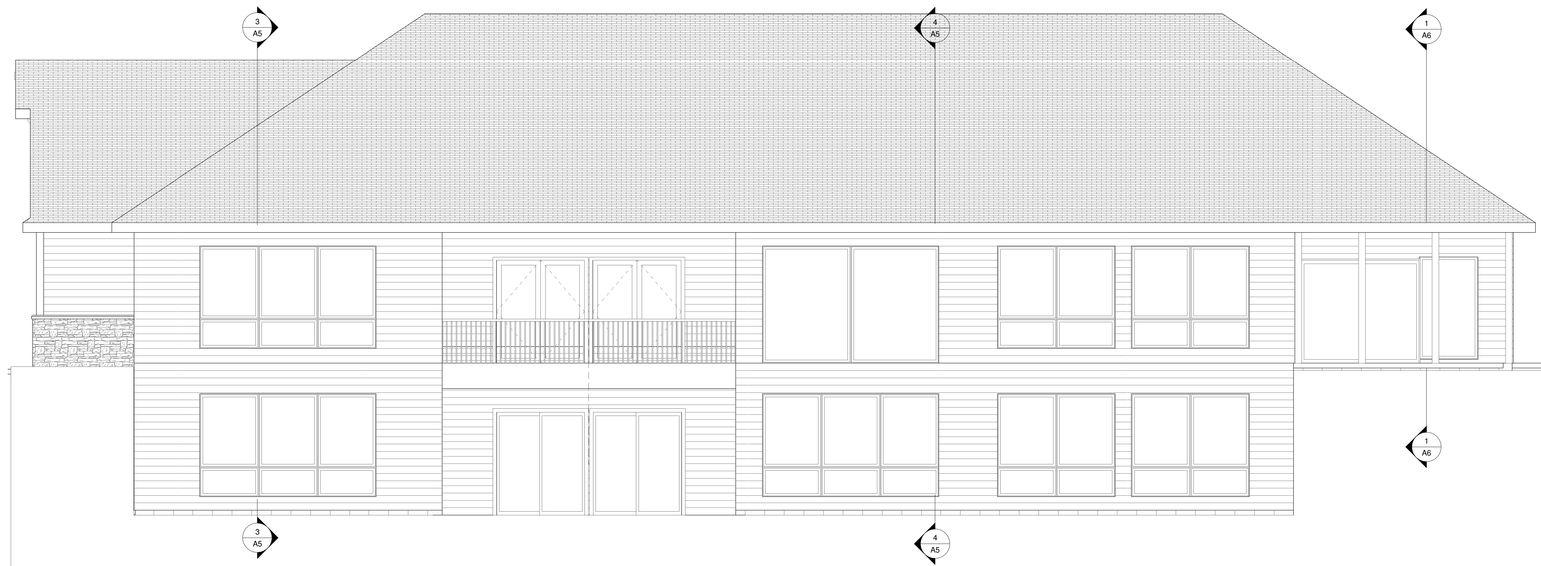
③ EAST EXTERIOR ELEVATION 1/4" = 1'-0"
