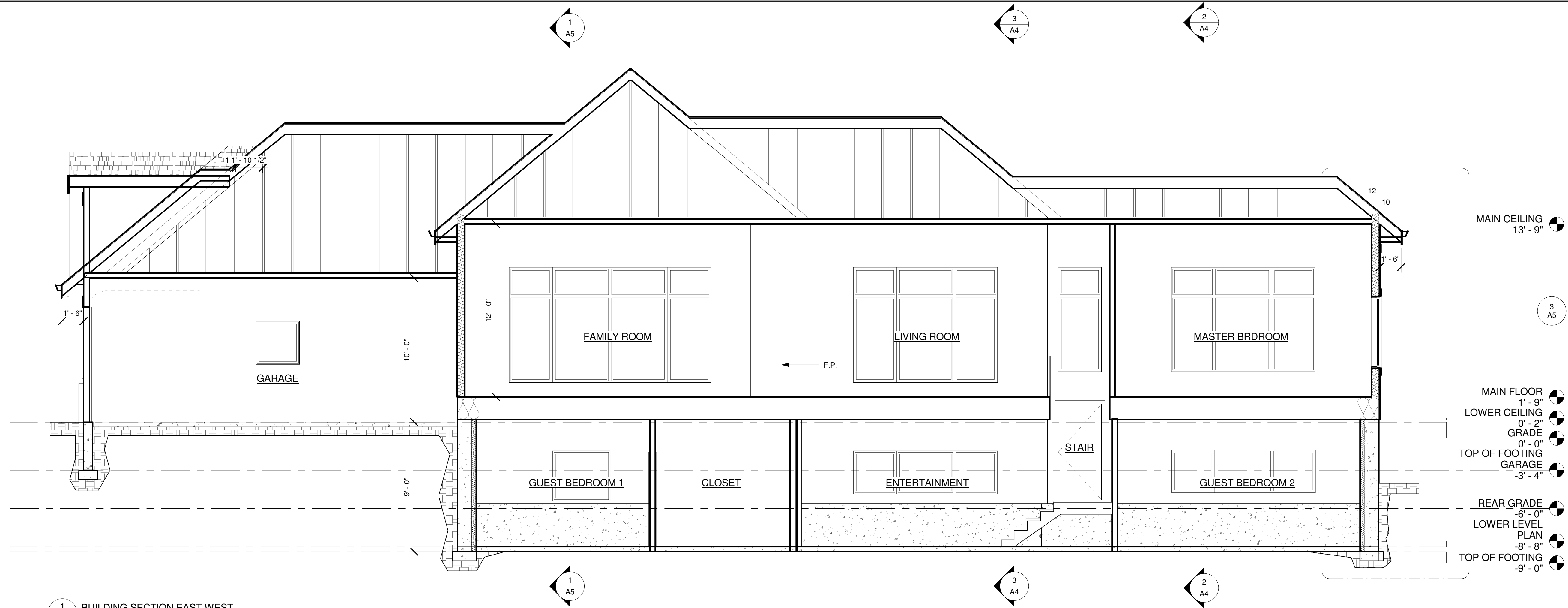
1 BUILDING SECTION EAST WEST A4 1/4" = 1'-0" SF:
