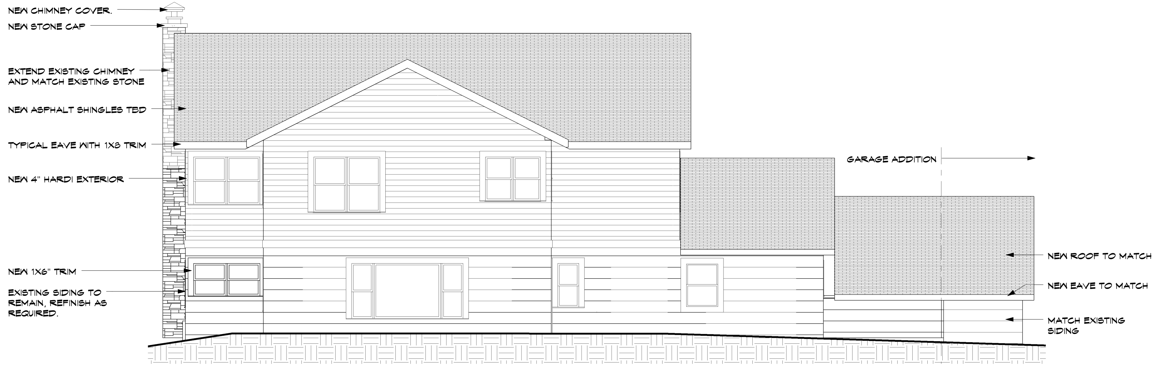
1 NORTH ELEVATION A5 3/16" = 1'-0"
